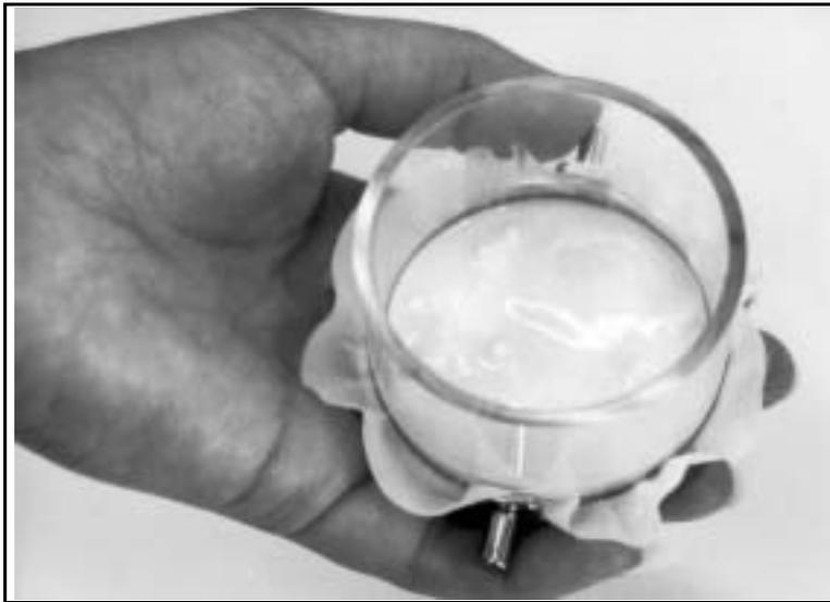
Fig. 7. Water spread evenly over the test sample.
