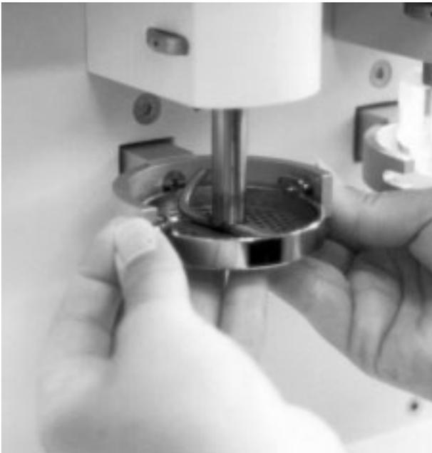
Fig. 16. Checking sieve - hook distance
