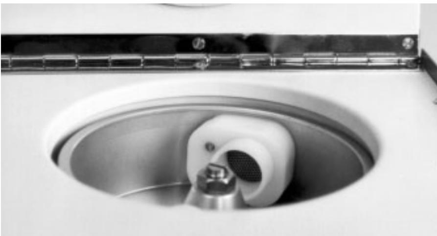
Fig. 5. Centrifuge cassettes in position.
