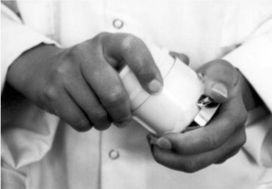
Fig. 4. Assembling the wash chamber. Fine sieve in the unmarked sieve holder.
