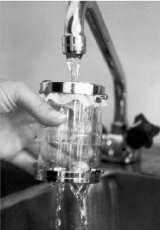
Fig. 8. Whole meal procedure. Transfer of partly washed out gluten.
