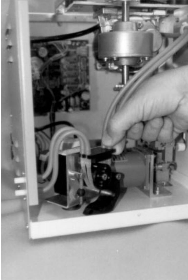
Fig 13. Releasing tube and nozzle from pump.
