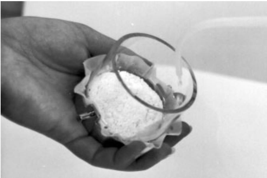
Fig. 6. Adding mix water to the sample. Water stream directed against the sidewall.
