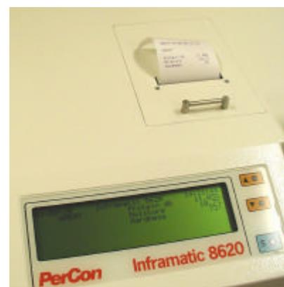
4. Open the sample compartment and clean out the sample using the soft brush supplied. Keep the sample window clean at all times. Should the sample window be contaminated with oil or fat residues these are best removed using a soft cloth moistened with alcohol or methylated spirits. Such cleaning may also be required between individual samples if the oil/fat content of the sample is high. For wheat, barley and wheat flour samples, cleaning with the soft brush is sufficient.
