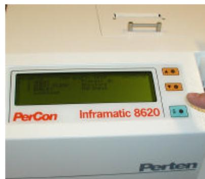
3. The analysis starts and when finished the result is presented on the display. If the instrument is equipped with a printer the results can be printed.
